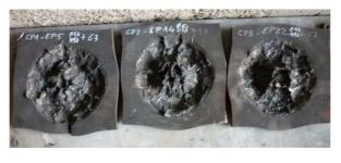
Figure 10: Recovery of the witness plates, test at +63°C
