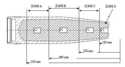
Figure 7: Strenght and chemical XF® block samples – localisation
