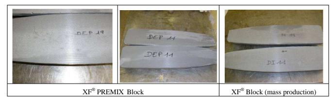
Figure 8: View of XF® PREMIX blocks after cutting
