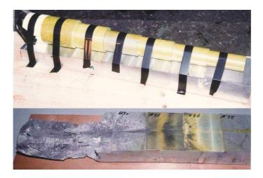
Figure 2: Critical Unconfined Diameter configuration (fig, top) and results (fig, bottom)
